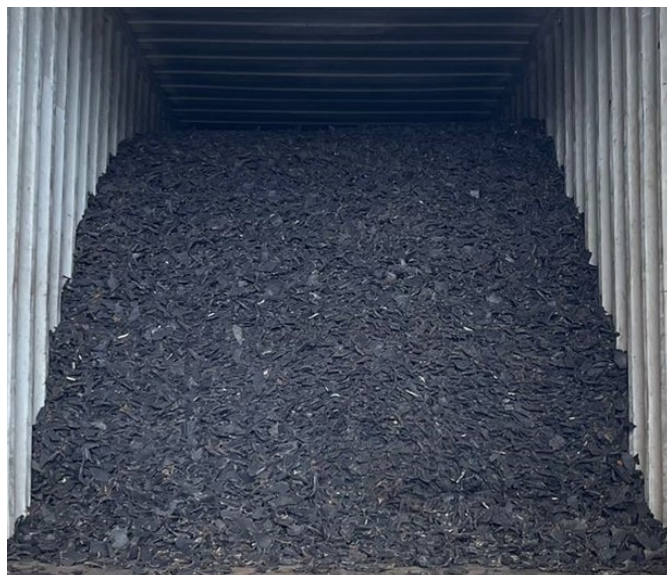
Stock photograph of shredded tires containerized for shipping Tire Processing facility. (Photograph courtesy of Guahan Waste).
